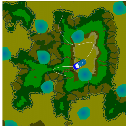
Figure 1: Motivating scenario: A ground vehicle needs to safely explore unseen environments to learn the effect of different terrains (in different colors) on its dynamics. The light blue regions are pools that the vehicle should avoid.
