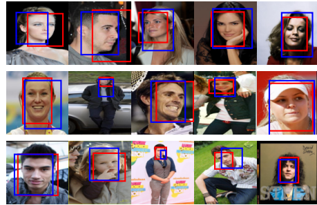
Fig. 6. Face detection on sample test images from CelebA dataset [87] using DAREK. Red boxes indicate ground-truth bounding boxes, and blue boxes indicate DAREK predictions. Note that it uses only 100 projected dimensions out of a 25k-dimensional feature space of ResNet18.
